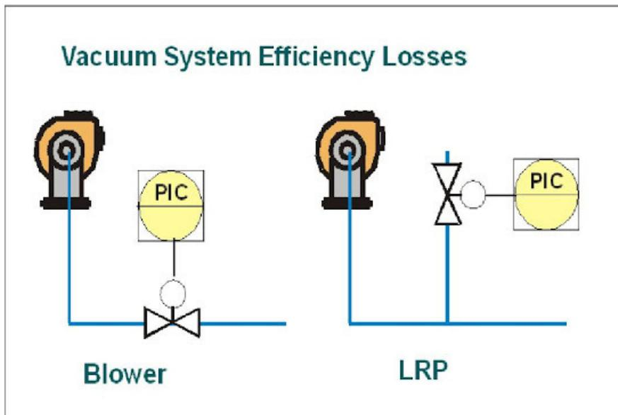
**Picture 3:** Vacuum level control principles.
