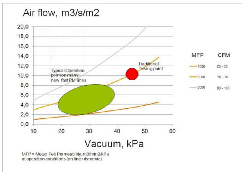
**Picture 1:** Operating conditions of felt conditioning.
